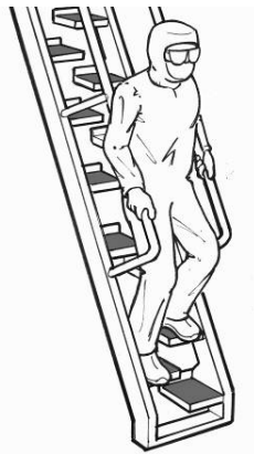
Figure RX-9 Descending an Alternating Tread Stair Ladder While Facing the Direction of Travel
